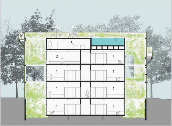
SCHEMATIC SECTION - HOTEL ANNEX (1) hotel rooms (2) sauna (3) technical room (4) swimming pool (5) external ramp to swimming pool access
