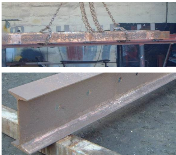
Figure 11: The trial cleaning on one of the transverse beams, before (above) and after (below).
