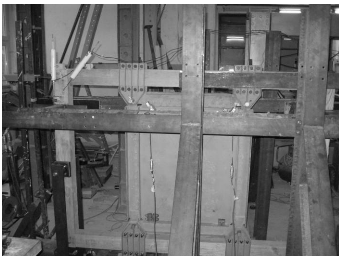
Figure 17. Test specimen of metal shear panels for consolidating timber structures.
