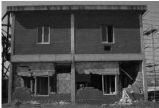
Figure 9. Damage in the real R.C. building after the test on the original structure without reinforcement.
